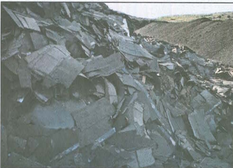
Asphalt shingles before and after. In the foreground, shingles awaiting processing will be turned into a raw material like that in the background.
