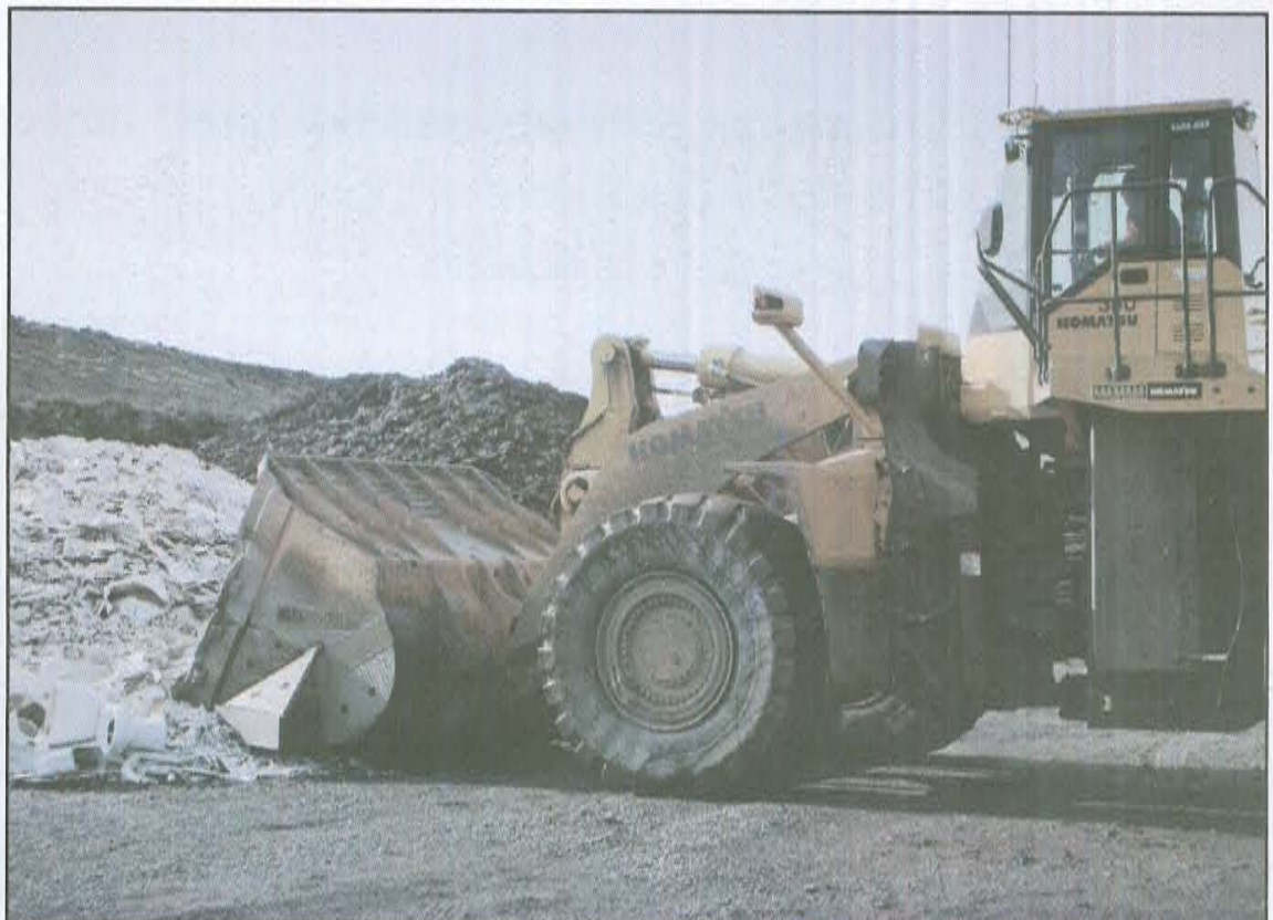
A loader prepares to move some of the porcelain recyclables to be ground into useful cement ingredients.
